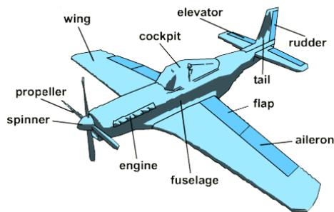
**Aileron** - Surfaces on the wing that moves up and down.
